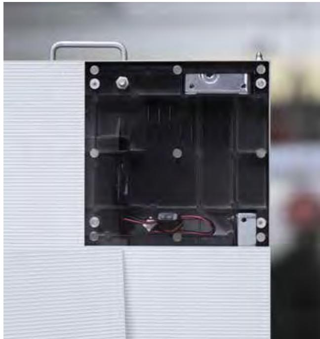
Modules are mounted via magnets. Just press the button from the back of the cabinet and detach the serviced module
