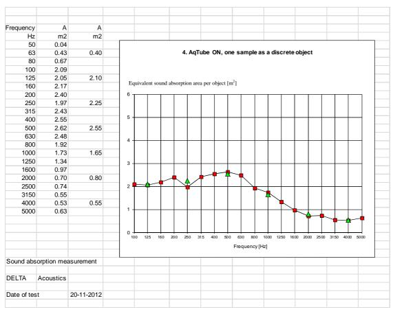
Equivalent sound absorption area per object for AqTube ON, double tube mounted as a discrete object, one sample, measured in two different positions.
