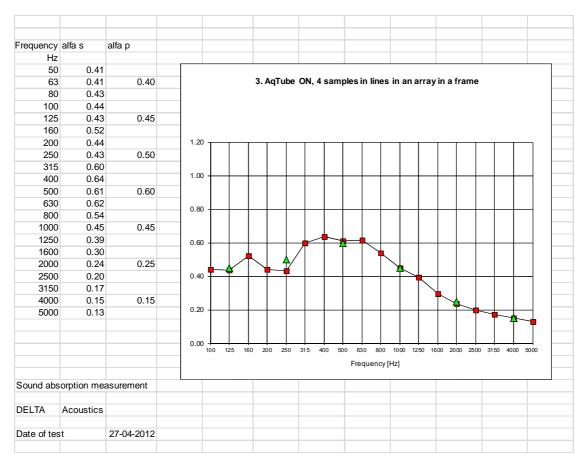
Sound absorption coefficient for AqTube ON, double tubes mounted in lines in an array in a frame (3.00 m x 3.33 m x 1.00 m), 4 samples, c-c 0.75 m.
