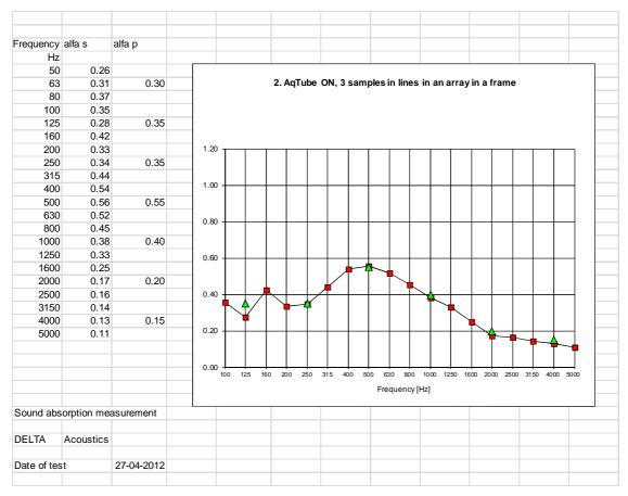
Sound absorption coefficient for AqTube ON, double tubes mounted in lines in an array in a frame (3.00 m x 3.33 m x 1.00 m), 3 samples, c-c 1.00 m.
