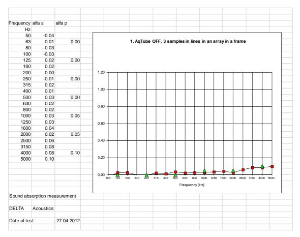
Sound absorption coefficient for AqTube OFF, double tubes mounted in lines in an array in a frame (3.00 m x 3.60 m x 1.20 m), 3 samples, c-c 1.00 m.
