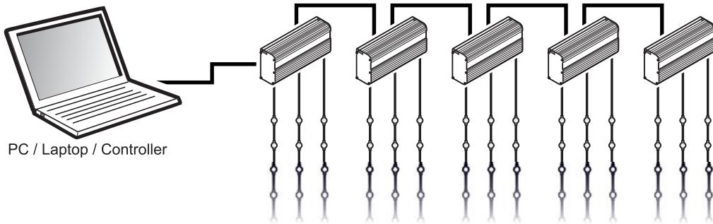
For communication to function, both the ILD and the PC must be on the same local area network (LAN) with IP addresses in the 2.x.x.x range (which are IP addresses used and recognised by Artnet). The PC can be connected directly to an ILD using a network Ethernet cable, and up to ILDs can be daisy-chained. To connect more than five ILDs, use an Ethernet switch, but do not connect more than five ILDs to each port.
