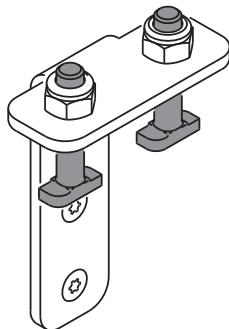
Use two T-Bolt Brackets to attach an ILD to a flat surface. These brackets are secured to the mounting surface using three pieces of M6 hardware. To attach an ILD to a bracket, slide the t-bolts into the attachment rail in the ILD casing (A), turn the bolt 90 degrees so that its head is under the rail rim, and then secure by tightening the nut (B).
