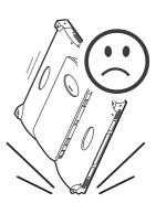
To avoid damage to the panels, it is recommended to leave the panels in the flight case until needed. Lift the panels one at a time from the flight case, using the handle on the back of the panel.
