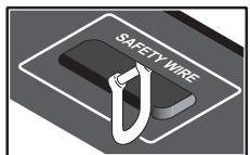
Fasten a safety cable (not shown) between the support structure and the attachment point on the fixture. The safety cable must be approved for a safe working load (SWL) of 10 times the weight of the fixture.
