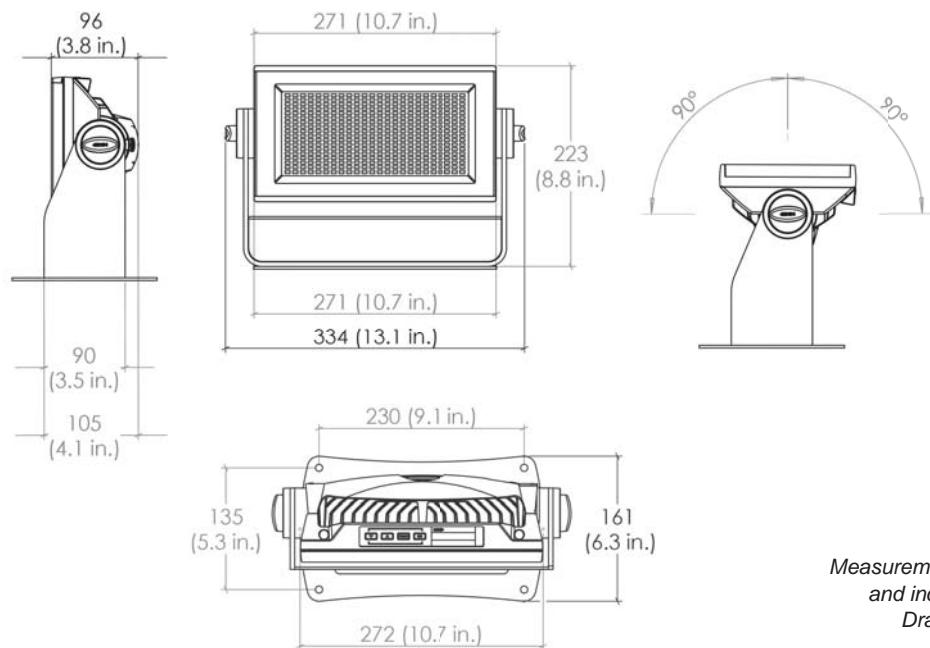
Measurements in millimetres
