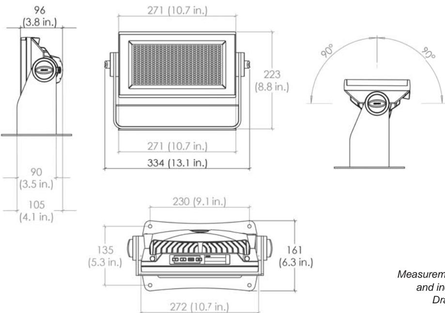
Measurements in millimetres
