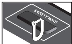
Fasten a safety cable (not shown) between the support structure and the attachment point on the fixture. The safety cable must be approved for a safe working load (SWL) of 10 times the weight of the fixture.
