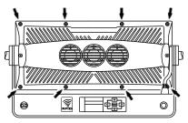
2 Dismantle the front and unscrew the highlighted front plugs with an Unbrako 6/HOP6 Allen key.
