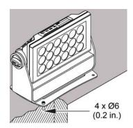
One Omega bracket is supplied with the fixture if it is to be flown above the ground. Remove the floor stand/base and rig the P-2 to a support truss or structure using the supplied brackets and suitable clamps.
