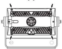
2 Dismantle the front and unscrew the highlighted front plugs with an Unbrako 6/HOP6 Allen key.
