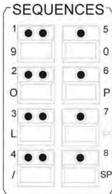
Eight keys are available in the Sequences section to select and store sequences. They can be switched with the Shift key in combination with the activated sequence key (with incorporated green LED).
