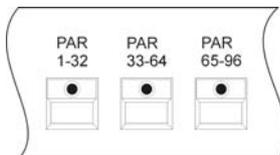
In order to gain direct access to the edit functions of the PAR section, one of the three PAR keys in the Feature Selection block must be pressed first.
