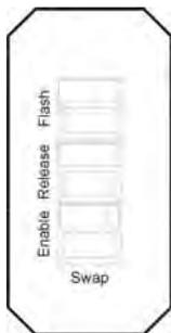
**FLASH:** Flash function of cue keys or chase keys (in combination with the release function). This function will only work in combination with an R-Link.
