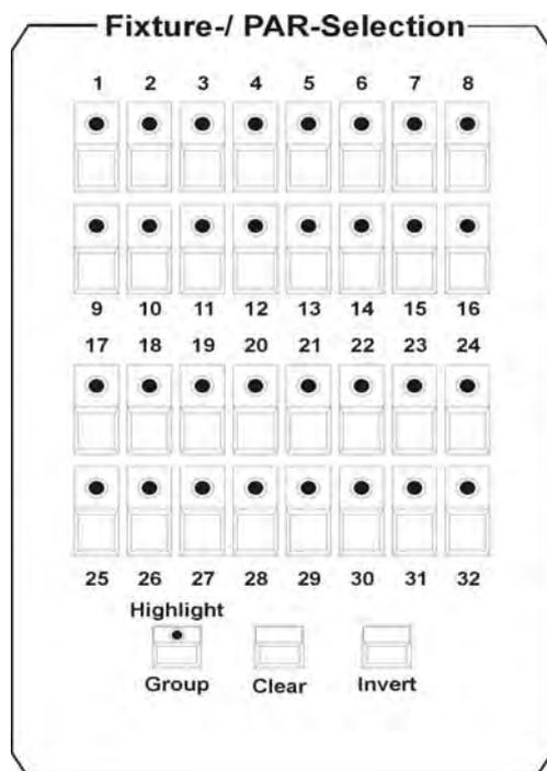
The Licon 1X allows access to a total of 32 fixtures. The fixtures are activated with the keys of the Fixture-/PAR Selection (keys 1-32). The fixtures are activated, when the corresponding LED is lit.
