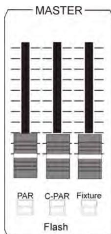
First of all press the GROUP key in the Fixture-/PAR Selection (the LED of the Group/Highlight key is lit). Then activate the stored groups by selection of the desired switch-keys 1-8 in the Fixtures section. The LEDs of the activated fixtures are lit.
