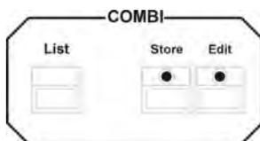
Confirm the process by pressing the Store key in the Combi section again.
