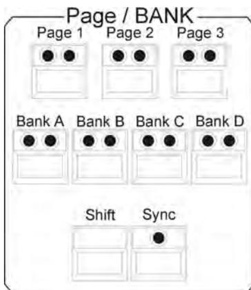
This block is used to switch the individual cue, chase and sequence keys.
