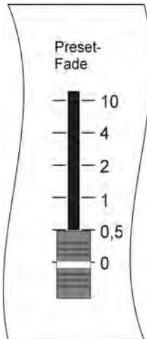
The fading of presets requires that the Preset-Fade fader is raised. This fader is located in the Feature Selection section (below the ON/OFF switch) and has a scale ranging from 0.0 seconds to 10 seconds.
