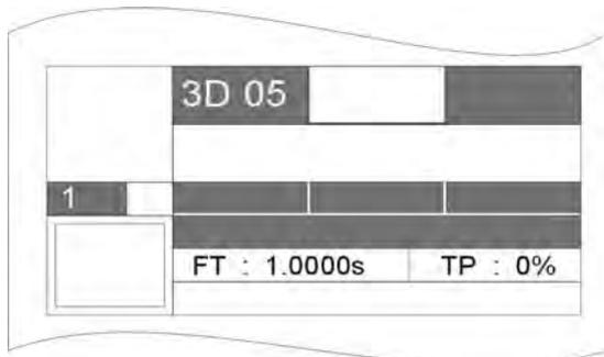
Each cue can be assigned a fixed fade time. This fade time accesses all parameters marked with a fade ramp in the storage matrix. It determines the speed, at which the corresponding features are faded in. Enter the fade time with the left encoder wheel (FADETIME). The maximum fade time amounts to 1638.3 seconds. The fade time is entered in one-tenths of a second.
