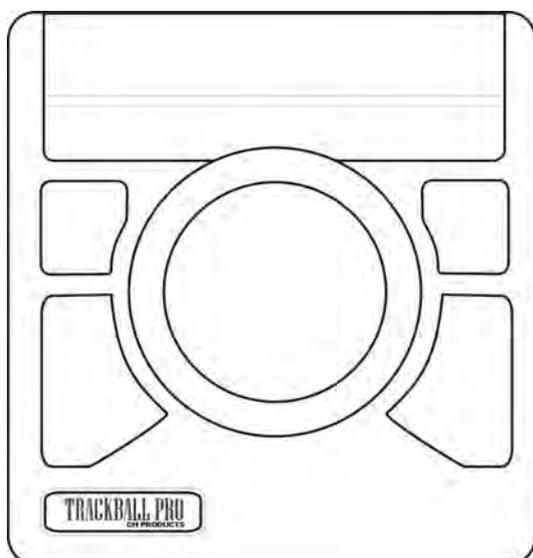
The trackball delivered by the manufacturer has 4 keys. The 2 smaller keys arranged above the big keys perform the same functions as the big keys.
