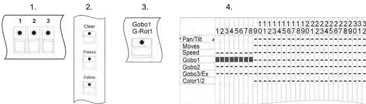
You can assign the freeze function to each feature available by newly defining the fixture selection and pressing the Freeze key once more in combination with the desired Feature Selection key.
