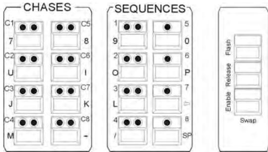
Use the Release-Link key to activate a release link. Together with the Flash-Release-Enable key, this key is located to the right of the Sequences block.
