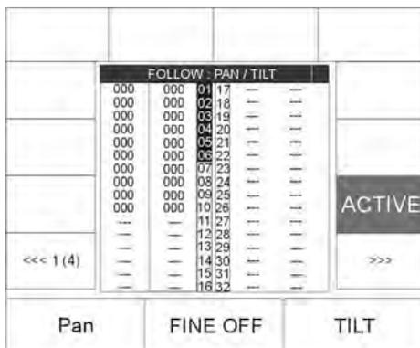
Activate the follow function by pressing and holding the Follow key in the Feature Selection block. The softkey ACTIVE appears on the display. Press this softkey to activate the follow function. The function field on the display is shown inverted when the function is active.
