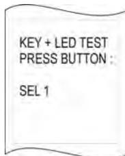
Press the softkey KEYS to test the function of the keys. The following display will appear:
