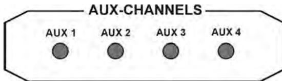
DMX devices such as fog machines can be assigned to the AUX controllers. These devices are controlled directly, irrespective of the other controller functions. The corresponding DMX output values are shown on the display in the main menu.
