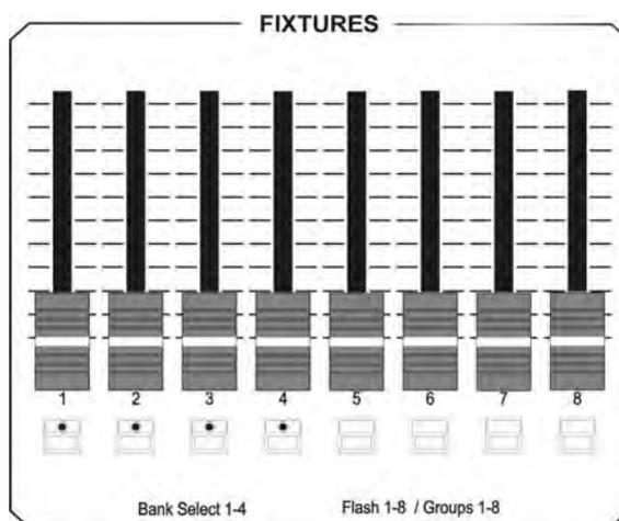
Use the 4 switch-keys with incorporated green LEDs in the FIXTURES section to switch the eight faders to four banks. In order to switch the banks, press and hold the SHIFT key and simultaneously press the desired bank (switch-key with green LED) in the FIXTURES section.
