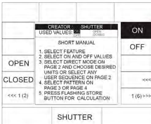
In the example on the left, the feature shutter is activated in the Feature Selection. (The display varies depending on the selected feature.)
