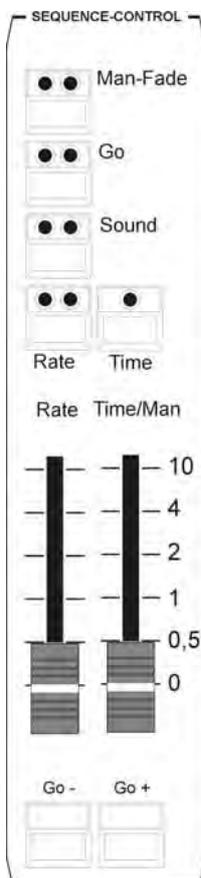
Each activated sequence will run according to the programmed runtimes and mode of flow control. However, it is possible to overwrite these times with the keys and faders of the Sequence Control section. The Sequence Control section has higher priority than the previously programmed data.
