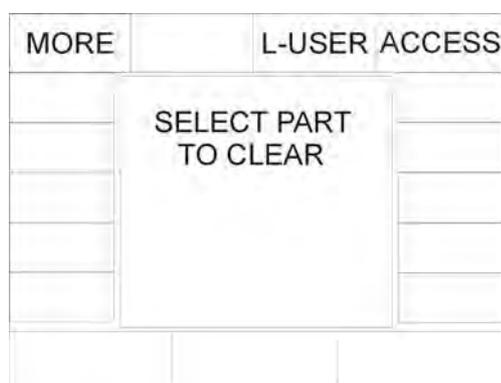
In this menu you can delete the self-programmed configuration of the fixtures or the assigned passwords.
