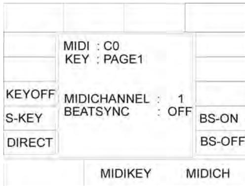
If the softkey DIRECT is displayed inverted also cues, chases and sequences can be assigned that are stored on the other pages and banks..
