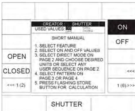
In addition, this page displays the presets that were previously stored for the activated feature (in our example for the shutter). You can select another feature by pressing the corresponding key in the Feature Selection block.
