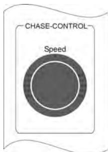
The duration of a step is entered with the encoder wheel (speed) in the Chase Control section.
