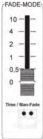
Whether or not you have assigned a fade time to your cues, you can activate a fade time with the Fade-Mode fader. The Fade-Mode fader has a higher priority than the fade times you have stored previously. The scale ranges between 0.0 and 10 seconds. The Time/Man fade key below has two incorporated LEDs.
