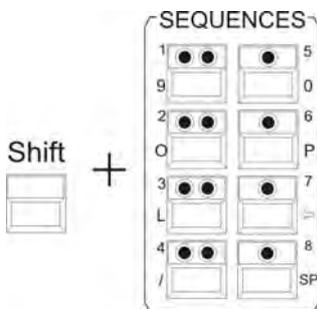
Press and hold the Shift key. Simultaneously press the desired bank key in the Sequences block (key with two LEDs). The green LED of the selected bank begins flashing. Now press the desired sequence key. As soon as a sequence is selected, both the red LED of the sequence key and the green LED of the bank key are lit.
