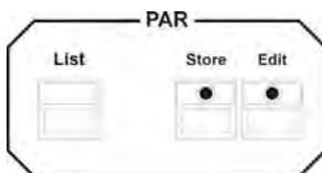
Select the desired PAR channels with the help of the individual programming functions (Chapters 18.1 to 18.6) and press the Store key in the PAR section (LED of Store key is lit). Then select a fader (1-8) in the PAR section and press the flash key located below this fader.
