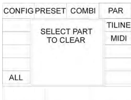
Select the desired section to be deleted by pressing the corresponding softkey and confirm with the softkey YES.
