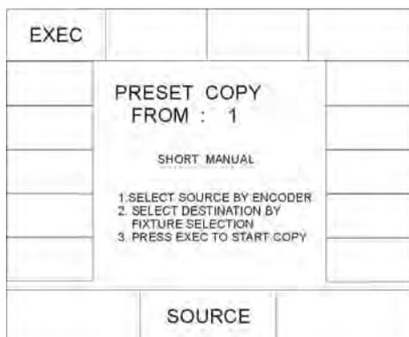
To enter the Preset Copy menu, press the softkey CONFIG in the main menu and afterwards the softkey P-COPY. Use the middle encoder wheel (SOURCE) to select the fixtures, the presets of which you want to use as source presets. Then select the keys of the fixtures in the Fixture-/PAR Selection (keys 1-32), to which you want to copy the presets.
