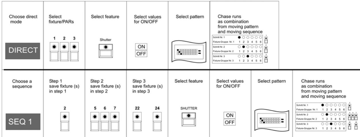
The chase runs as a combination of a fixture sequence and a chase pattern.
