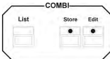
The Combi section performs all storage and edit functions for cues (scenes), chases and sequences, which contain either only fixtures or fixtures and PAR channels. In addition, all presets for fixtures as well as for PAR channels are stored by means of the keys of the Combi section.
