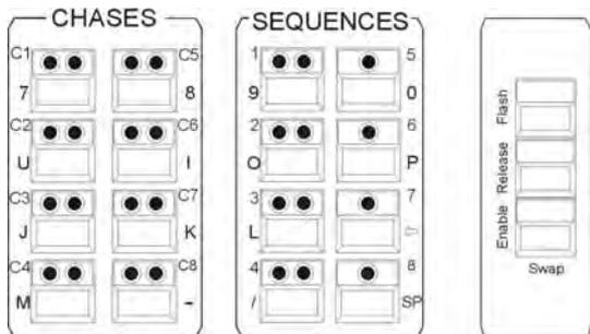
Working with the flash function is **only** possible, when a release link was assigned before! The flash key (as well as the release key and enable key) is located in the block right to the Sequences section. The release link can be assigned in the Combi Store or Combi Edit section according to the procedure described in Chapter 6.1.7.
