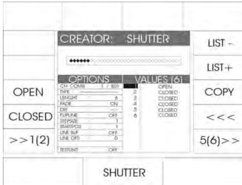
A standard chase always switches between two parameters (presets or DMX values). On Page 5 of the chase generator, you can extend the list of parameters to be assigned to a chase.
