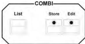
Enter the Edit menu by pressing the Edit key (LED is lit) in the Combi section. Select the desired cue by pressing the corresponding cue key and press the softkey MODIFY. You can now edit the individual parameters.
