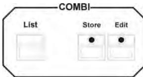
Press the Store key in the Combi section (the Store LED is lit) and press the corresponding softkey to select the desired storage place on the display (the Store LED is flashing).
