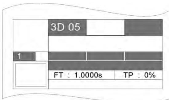
A trigpoint can be assigned to all switchable features. It designates the moment, at which all parameters that cannot be faded are switched. This applies e.g. to gobos, prisms, etc.
