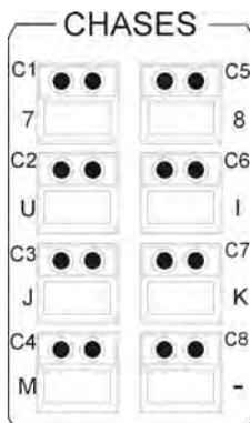
The Licon 1X has a total of 94 storage places (keys) for chases. 32 chases can run at the same time.
