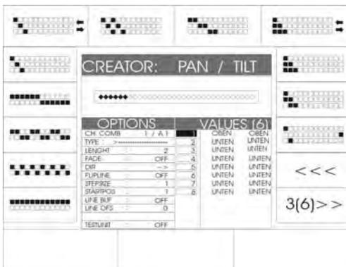
A variety of chase patterns is available here. They can be activated with the corresponding softkeys. On the display, a graph illustrating 32 fixtures is shown. The inverted fields in the graph indicate activated fixtures.
