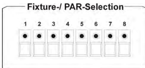
Press and hold the no. 8 in the Fixture-/PAR Selection of the Licon 1X in the OFF-state of the console and simultaneously turn the console on with the ON/OFF key.
