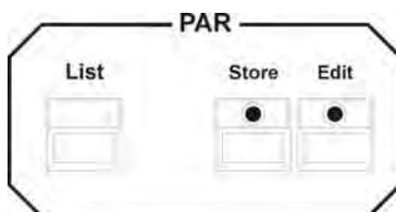
The PAR section performs all storage and edit functions for cues (scenes) and chases, which only contain PAR channels and which are activated by the PAR faders.
