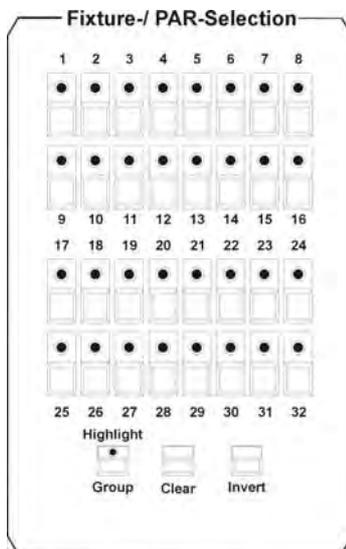
The keys 1-32 are used to activate fixtures or, in combination with the PAR keys, to activate PAR channels.
