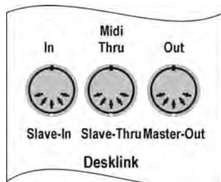
MIDI devices are connected to the Licon 1X with a standard 5-pin MIDI cable. The MIDI sockets are located on the rear panel of the Licon 1X. Connect your MIDI cable to the MIDI-In socket of the Licon 1X and to the MIDI-Out socket of your MIDI device.
