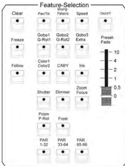
The freeze function is used to lock fixture parameters.
