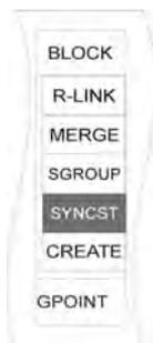
The softkey SYNCST is displayed, when a chase is assigned to a speed group during the storage process.
