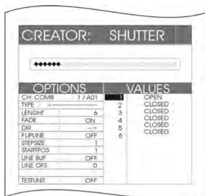
When you have selected the number and sequence of the desired fixtures or dimmers, press the corresponding softkey to select the desired chase pattern. The display will immediately show the number and the sequence of the chase steps.
