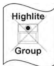
In order to flash the moving heads of a fixture group, press and hold the Highlite/Group key (LED is not lit) and simultaneously press one of the flash-keys located below the fixture faders. Then release both keys again.
