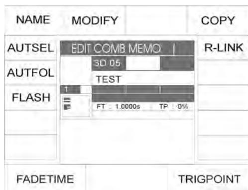
Press the corresponding softkey to activate the AUTSEL function. When the function is active, the softkey is displayed inverted.
