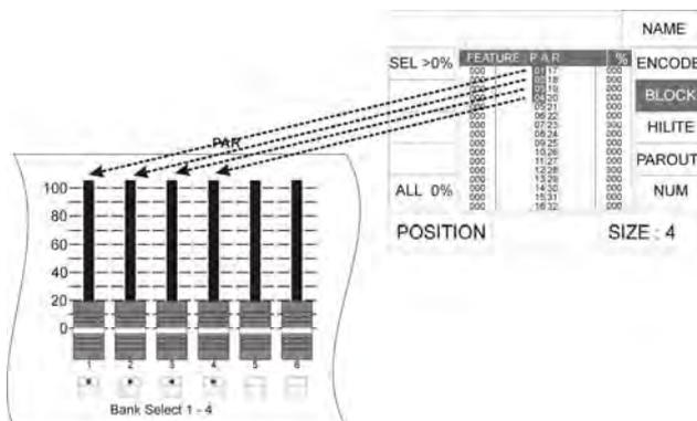
Since the DMX values of a channel are entered with the 12 PAR faders, a maximum of 12 PAR channels can be assigned to a block. You can change the position of a block with the left encoder wheel.
