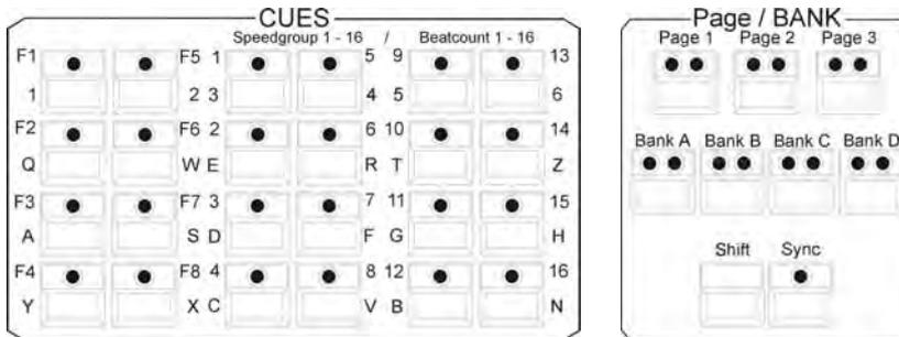
On each key of the first block (each key is labelled with a number from F1 to F8), a single cue can be stored. This block is reserved for important cues that are often activated. The cue keys of the first block cannot be switched with the Page/Bank function.
