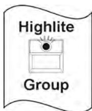
There are two different ways of working with the group function: Press the Highlite/Group key (LED is lit). Now you can activate fixture groups that have been previously stored on the fixture faders. Press the flash-key located below the corresponding fader. If the master fader and the fixture fader are raised, the fixtures integrated in the corresponding fixture group are lit.
