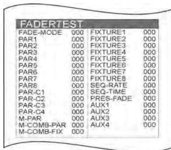
Activate the Test menu as described in Chapter 21.8.1 and press the softkey FADER. The display shown on the left appears:
