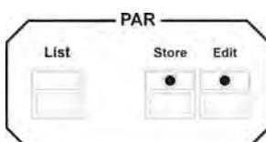
Select the desired PAR channels with the help of the individual programming functions (Chapters 18.1 to 18.6) and press the Store key in the PAR section (LED of Store key is lit). Then select a fader (C1-C4) in the PAR section and press the flash key located below this fader.
