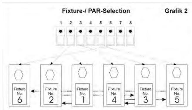
However, this mode cannot be applied to all stage settings, since the fixtures are often not arranged according to their sequence in the Fixture/PAR selection (see Fig. 2) or sometimes more than one fixture (-> a fixture group) should be addressed.
