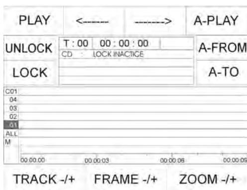
Before a CD can be inserted, you must unlock the CD drive by pressing the softkey UNLOCK. The display will confirm with the message LOCK INACTIVE. Open the CD drive by pressing the key located at the disk tray and insert a CD. We recommend locking of the CD drive after insertion of the CD, so that you cannot open it by mistake during use. Press the softkey LOCK to lock the CD drive again. The display confirms the process with the message LOCK ACTIVE.
