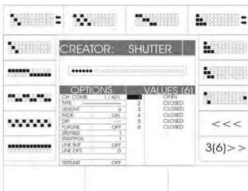
A total of 24 chase patterns are available on pages 3 and 4 of the chase generator. These are selected with the corresponding softkeys and combined with the fixture sequence programmed previously.
