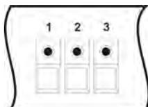
Then press and hold the STORE key in the Combi section and simultaneously press the switch-key in the Fixture section (keys below the fixture faders), on which you want to store the fixture group (choose between switch-keys 1-8). Then release both keys again.
