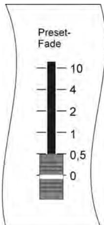
Press one of the PAR keys in the Feature Selection block. The stored Presets will be shown on the display and can be recalled with the corresponding softkeys. The fading time of PAR presets is controlled with the Preset-Fade fader in the Feature Selection block. Select a fade time between 0.0 to 10 seconds.
