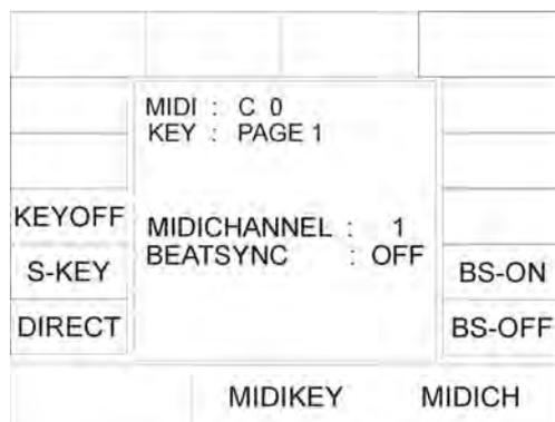
16 different channels are available for MIDI. The Licon 1X will only react to MIDI commands that are received on the selected channel. Press the softkey CONFIG/MIDI to enter the corresponding menu. Use the right encoder wheel (MIDICH) to enter the MIDI channel. The corresponding MIDI channel is also shown on the display (see illustration on the left).
