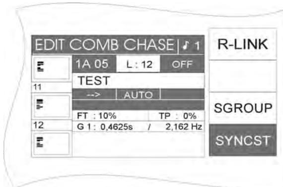
The softkey SYNCST is displayed, when a chase is assigned to a speed group in the Edit Combi Chase menu.
