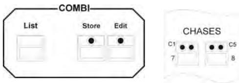
In the Edit Combi Chase menu, the function SGROUP is displayed. Press and hold the softkey SGROUP. Simultaneously press one of the speedgroup keys in the Cue section, to which you want to assign the chase.
