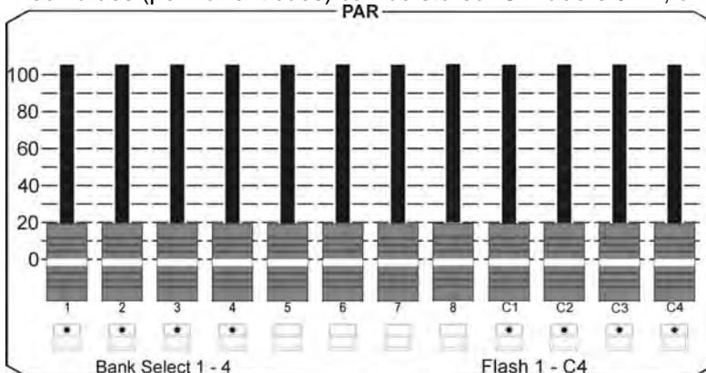
These 12 faders can be switched four times by the key combination „SHIFT + Flash keys 1-4 (green LED). Thus a total of 48 faders can be used to store PAR channels.
