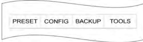
Enter the main menu, press the softkey BACKUP and select the function FORMAT. Confirm the process by pressing the softkey YES.
