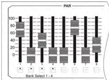
Brightness output in the Fixture-/ PAR Selection is controlled with the corresponding faders. If the swap key is pressed simultaneously with the flash key located below a fader, then the brightness output of all other faders is set to zero. Only the values of those fader(s) with activated flash keys will be output. Depending on the CONFIG settings, the swap function accesses the PAR faders, the fixture faders or both fader banks.
