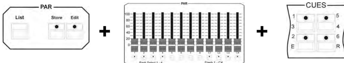
Press and hold the Store key in the PAR section. Select a PAR fader and press the flash key located below this fader. Then press the Cue key, on which the desired cue is stored. Release the Store key again and the cue is linked to the fader.
