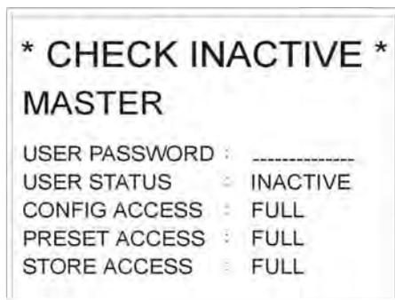
Enter the CONFIG menu and press the softkey ACCESS. The display shown on the left appears.
