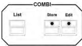
With the List function, you can have all named cues, chases and sequences shown on the display. This function is activated with the List key in the Combi or PAR section.
