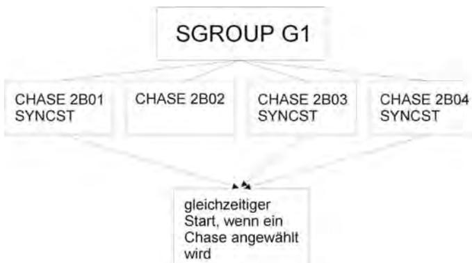
The Synchronised Start function has the same visual effect as the MERGE function, although they are managed differently by the lighting control console. Whereas the MERGE function is a fixed connection between two or more chases, which cannot be dissolved so easily, you can delete the Synchronised Start function with only one keystroke.
