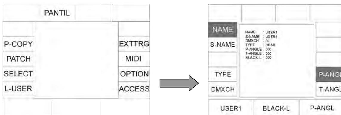
With the left encoder wheel you can select up to 20 different L-User fixture parameters.
