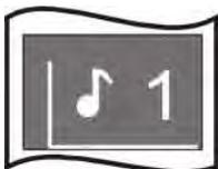
On the display, the number to the right of the note sign indicates the number of the bass beats that must elapse before the chase or sequence is switched forward by one chase step. In this example, the next chase step is recalled after one bass beat. Recall the sound function by pressing the Edit key or the Store key in the Combi section simultaneously with the chase key.
