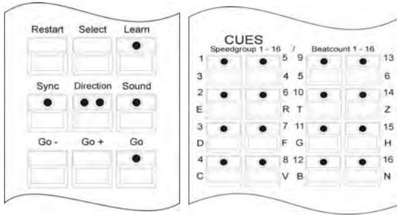
In the Prog Chase or Edit Chase menu, you can enter the number of bass beats by simultaneously pressing the Sound key in the Chase Control section and one of the beat-count keys in the Cues section.
