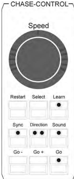
Encoder-wheel (SPEED): for manual speed regulation.
