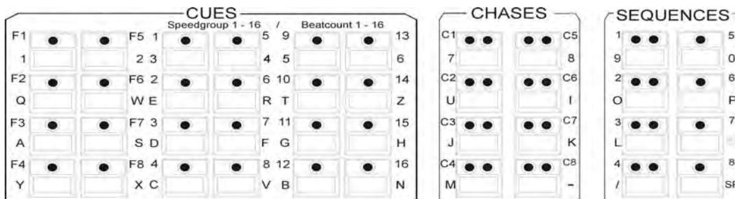
Before a preset is stored, you can name it with the double-assigned keys of the Cues/Chases/Sequences section. (For this purpose, a letter of the alphabet is assigned to each of these keys. The letters are arranged as on a conventional PC keyboard.) Confirm the entry with Store.
