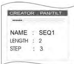
Each newly programmed step is added to the other steps. You can see on the display, how many steps you have already programmed. The number of steps of the sequence already programmed is displayed after the designation LENGTH. STEP on the display indicates the step, which you are currently programming.
