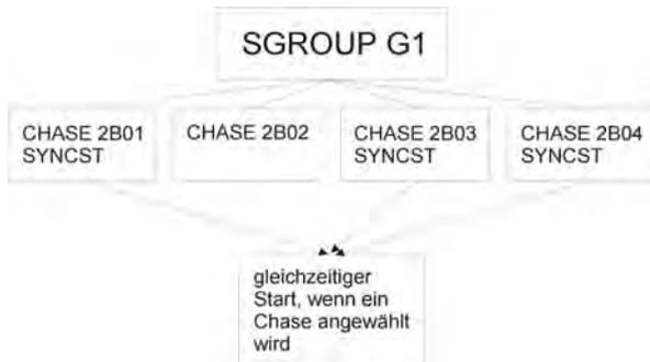
All chases of a speed group, to which the **Synchronised Start function (SYNCST)** is assigned, will start collectively, when one chase of the group is activated.
