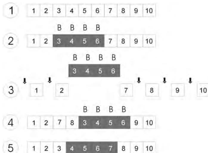
Define a block as described above. Moving a block does not mean that this block is duplicated (see: Copying a block). Your block is only moved to another position within the chase. The block is always inserted before the step that you have selected with the cursor.
