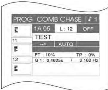
In the middle part of the display, the name of the speed group is shown, to which the assignment of the chase was made (here: speed group 1 (G1)). In addition, another function appears on the display, i.e. the Synchronised Start function (SYNCST).
