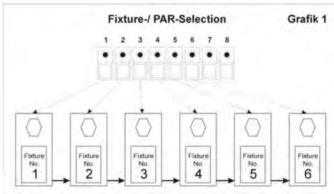
If a chase pattern is programmed in the DIRECT mode, the fixtures are always recalled according to the sequence of the keys in the Fixture/PAR selection (see Fig. 1). Every chase step addresses only one fixture.
