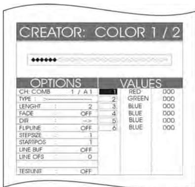
In this example, the colour green was added to chase step 2. The chase is now structured as follows:
