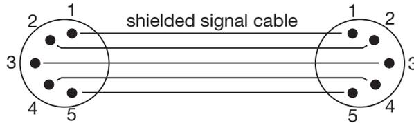
The P4 has 3pin and 5pin XLR connectors for DMX-in and DMX-out. Do not connect more than one data input and one data output on a fixture.
