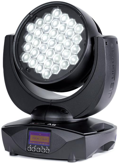
**A8 Tunable White.** The power-pack A8 is now also available with white LEDs. It is equipped with 37 multi-chip LEDs in the 15W class. Each multi-chip LED has two cold-white and two warm-white chips, which allow continuous adjustment of the colour temperature from 2900 Kelvin to 7700 Kelvin.
